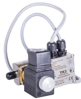
Designed to control the oil level in the compressor crankcase in order to avoid the compressor to run without oil and so improve its lifetime. TK3 monitors the oil level with the embedded electro-optic sensor and comprises a solenoid valve for oil filling and a relay output contact to give an alarm.
