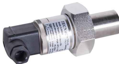
The optical level switch has been designed for use in level monitoring applications for the control of low viscosity liquids. It comprises an optical sensor and an output switch. It is realized in two parts to let it possible to replace the electronics without the needing of emptying or depressurizing the plant.
